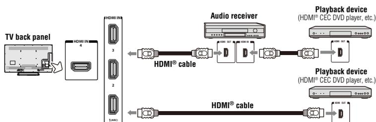
*(Sample Illustration) L7400U Series—Connecting an HDMI® CEC compatible audio system and playback device*
