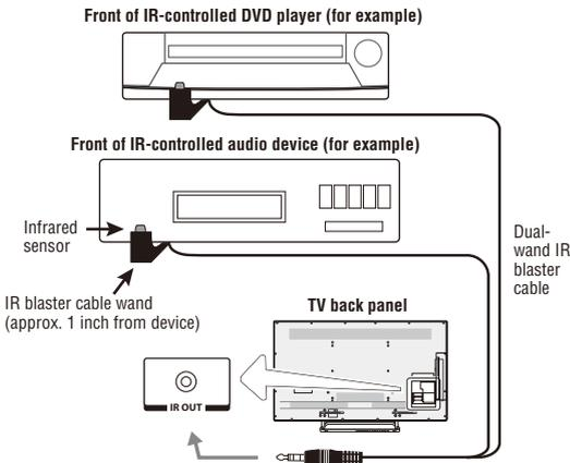
**(Sample Illustration) L7400U Series—Using the IR blaster OUT terminal**
