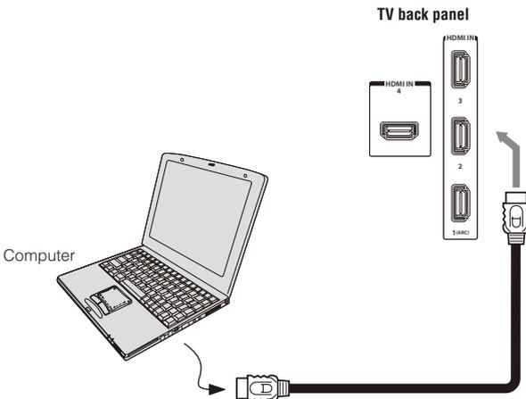
*(Sample Illustration) L7400U Series—Connecting to an HDMI® terminal*
