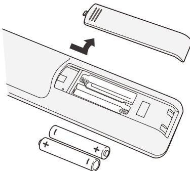
*(Sample Illustration) Removing the battery cover*
