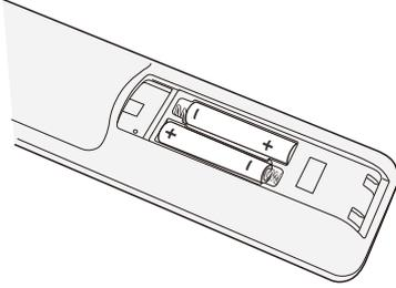
*(Sample Illustration) installing the batteries*
