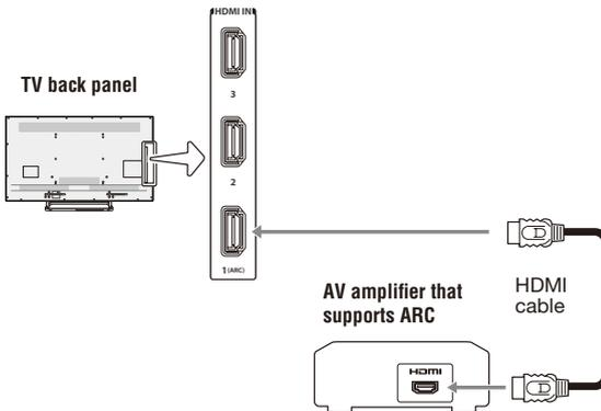
*(Sample Illustration) L7400U Series— Connecting to HDMI® ARC*
