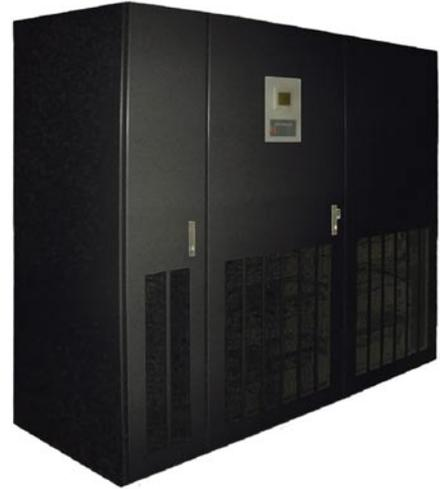
Using Toshiba IGBT technology in the rectifier/converter, DC/DC chopper, and inverter sections, the new models' double-conversion topology provides an AC/DC/AC efficiency of 97% at loads from 50% to 100%. Even at 20% loading, the efficiency remains greater than 95%. This industry-leading performance makes the G9000 the perfect solution for N+1 parallel systems where loads are typically 30 to 40%.
