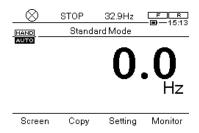
Enable a Forward run command. Increase your frequency reference above the lower limit value.
