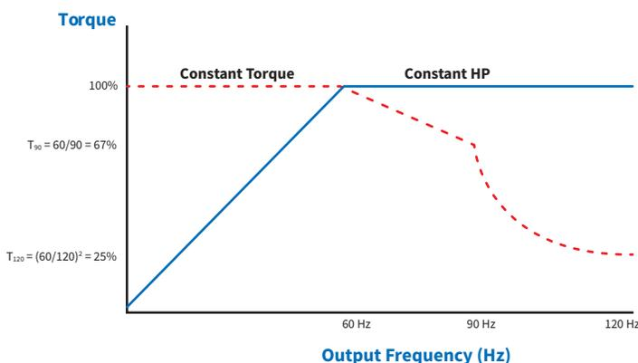
A 3 HP, 575 V drive was used to run a 3 HP, TEFC, 4-pole motor at 60, 90, 120, and 150 Hz. At rated motor current, the following maximum continuous torques were developed:
