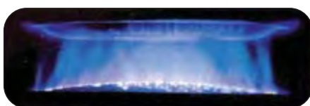
Axial Magnetic Field Interrupter - Arc Dispersion
