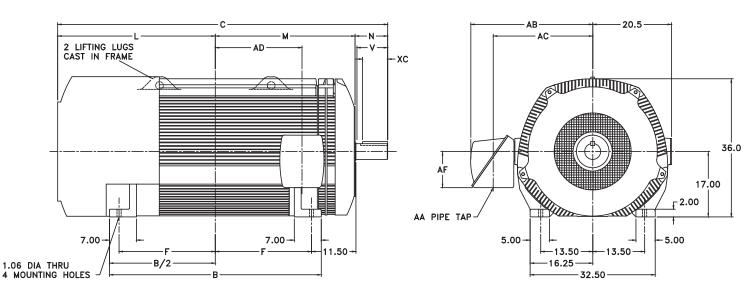
TYPE HS SQUIRREL CAGE INDUCTION MOTOR ENCLOSURE — TOTALLY ENCLOSED FAN COOLED AND EXPLOSION PROOF BEARING - ANTI-FRICTION AND SOLID SLEEVE
