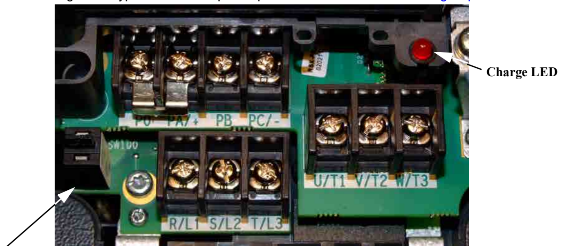
Figure 2. Typical G9 ASD Input/output Terminals and the Grounding Capacitor Switch .
