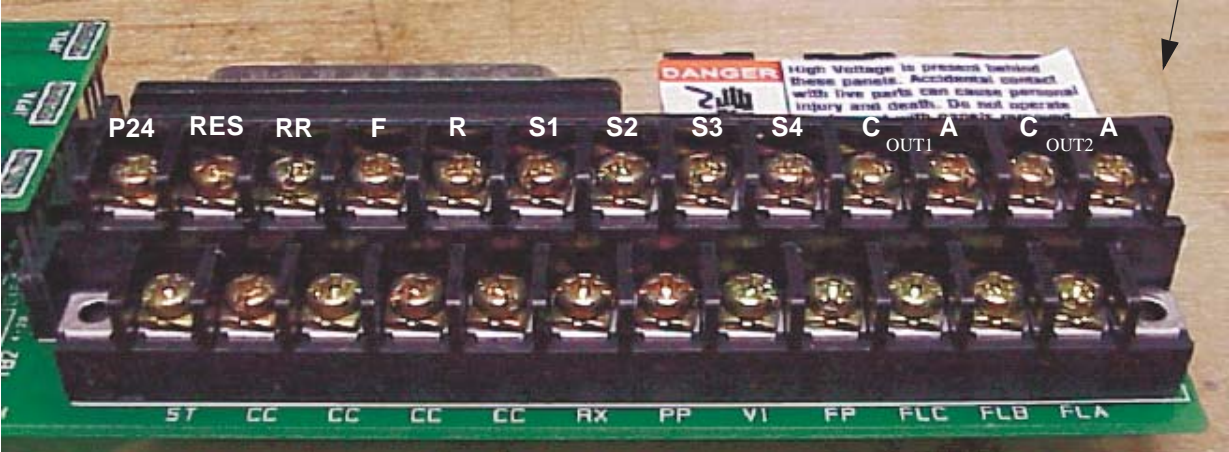
TB1 input and output terminals of the Terminal Board.
