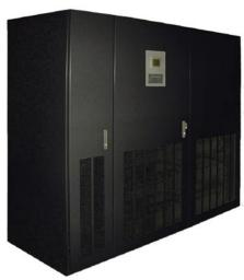
Using Toshiba IGBT technology in the rectifier/converter, DC/DC chopper, and inverter sections, the new models' double-conversion topology provides an AC/DC/AC efficiency of 97% at loads from 50% to 100%. Even at 20% loading, the efficiency remains greater than 95%. This industry-leading performance makes the G9000 the perfect solution for N+1 parallel systems where loads are typically 30 to 40%.
