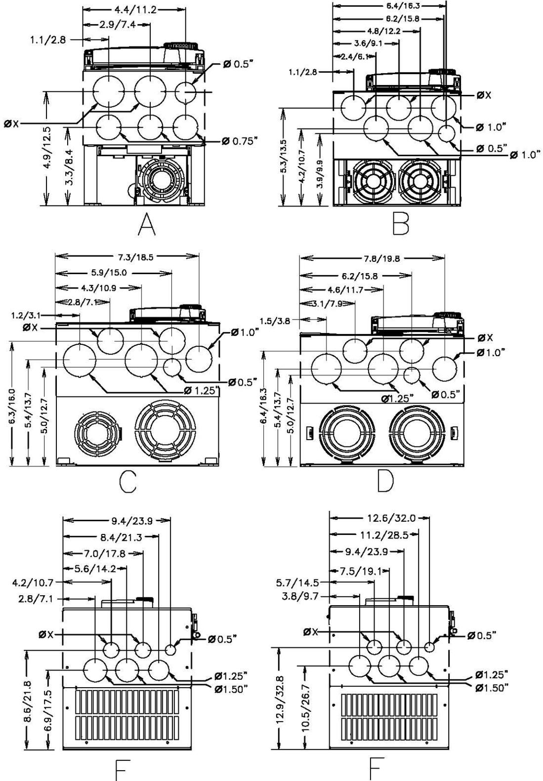
ØX = Concentric Knockouts for Diameter Sizes 0.5", 0.75", and 1.0" Conduit.
