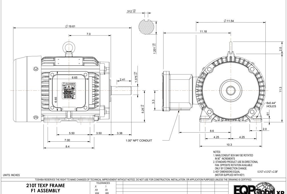
.XXX.005 XXXX. .0005 XT SERIES MDSLV800-03 MOTOR WEIGHT M. O'DOWD DRAWN BY: CHANGE T-BOX ASSEMBLY AND FAN COVER MO 03/24/14 JR CHECK BY: J. RUSSELL 221 lbs. FIRST ISSUE (OVERRIDE 'S' DIMENSION) MO 03/06/14 JR APPROVED BY: 101 kgs. **TOSHIBA INTERNATIONAL CORPORATION** NO DRAWN BY DATE CHECK REVISION www.toshiba.com/ind
