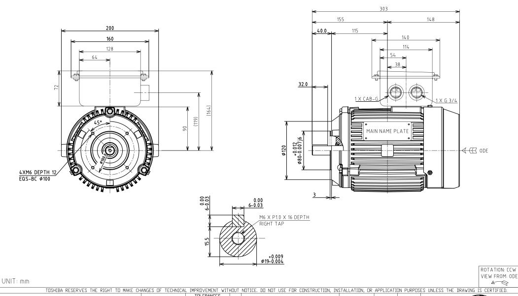
TOLERANCES B14-FLANGE MOTOR TYPE: 2-4-6P - 400V ±2.0 OL DRAWING IEC GLOBAL X.X ±0.5 FRAME: 80M X.XX $\pm 0.1$ 3HFN000313 MAXIMUM MOTOR WEIGHT HIEN. NGUYEN DRAWN BY: B.X.QUYNH CHECK BY: - lbs. 01 ND Change to P dimension and KEY length T.Danh Sep-10-18 B.Quynh APPROVED BY: JAY BUGBEE - kgs. TOSHIBA INTERNATIONAL CORPORATION REVISION DRAWN BY DATE CHECK www.toshiba.com/ind
